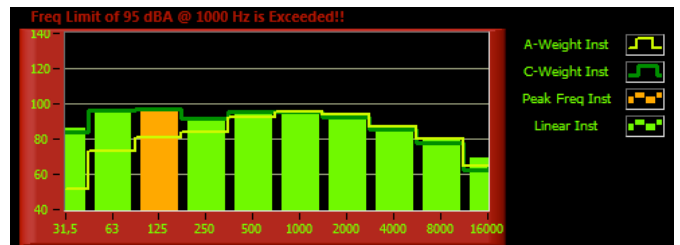
RTA limit monitoring is on – current value exceeds limit - notice that the actual limit violation is at 1 kHz, while the loudest frequency is at 125 Hz
