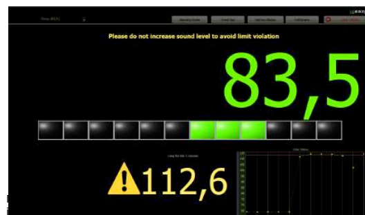
A flashing warning is triggered – Risk of limit violation if level is not reduced to a level where only green squares are lit.
