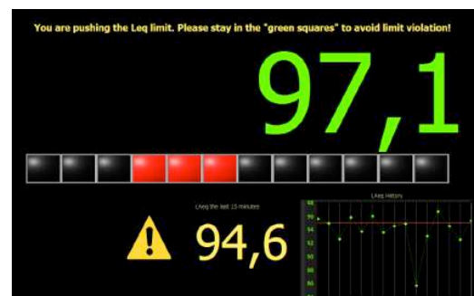
A flashing warning is triggered – Risk of limit violation if level is not reduced to a level where only green squares are lit.
